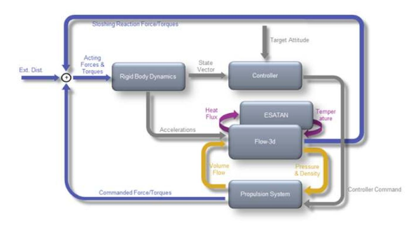
Multi-disciplinary simulations using coupled simulation (ESATAN, Flow3D,
