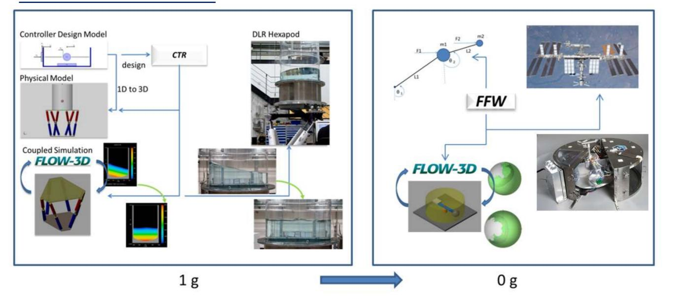
Modelling of sloshing usging the Bodel Based Design approach, based on MATLAB® and Simulink®.
