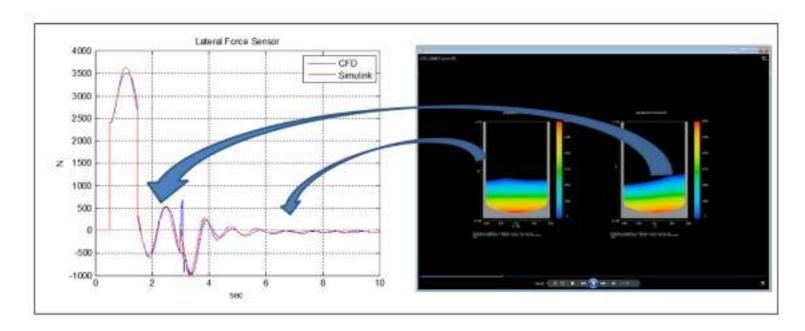
Closed-loop sloshing control to counteract sloshing and open-loop input shaping to avoid/reduce sloshing effects.
